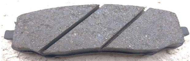
Fig. 10. Brake Pads after Wear Experimentation
