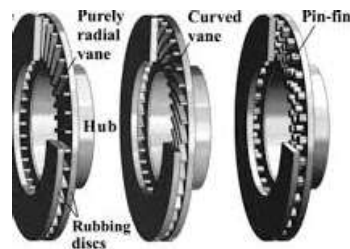
Fig 1. Friction disc of brake and different types of vanes on ACD brake disc
